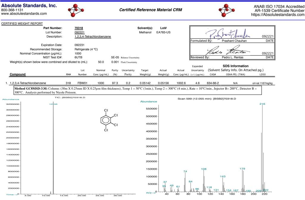
• The certified value is the concentration calculated from gravimetric and volumetric measurements unless otherwise stated.
